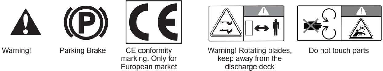
Warning!                  Parking Brake                  CE conformity marking. Only for European market                  Warning! Rotating blades, keep away from the discharge deck                  Do not touch parts
