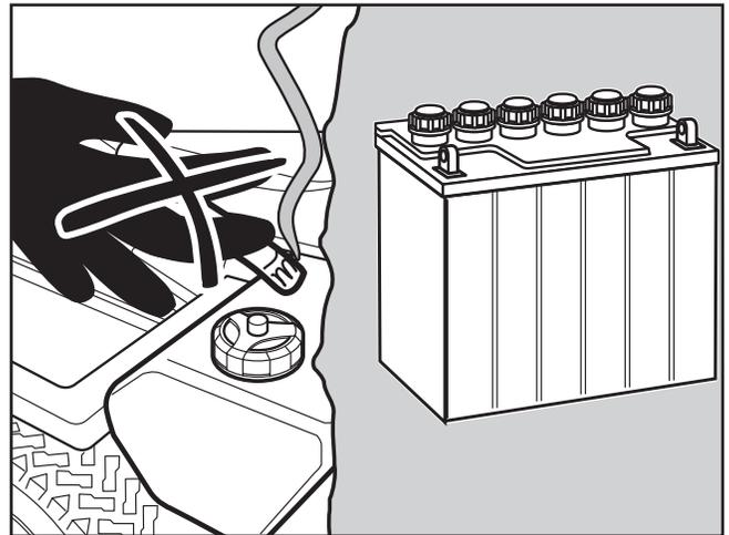
*Do not smoke when performing maintenance on the battery. The battery can explode and cause serious injury/damage.*
