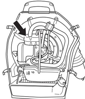
The muffler is equipped with a special spark arrester screen. The spark arrester screen should be cleaned once a month. This is best done with a wire brush.
