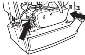
The air filter is fitted in the air filter cowl.
