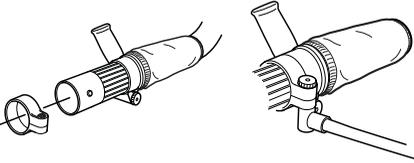
Assemble the intermediate pipe.
