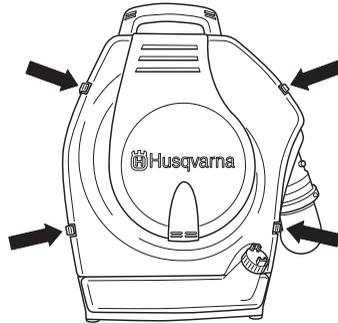
Loosen the two fasteners holding the air filter cowl and remove the filter. Wash the filter clean in warm, soapy water.
