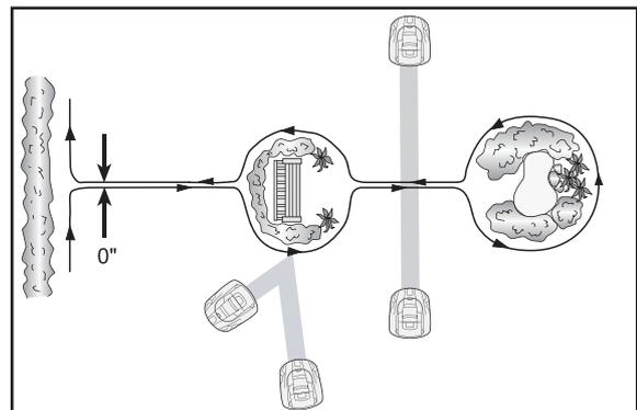
Obstacles that can withstand a collision, for example, trees or bushes higher than 6" (15 cm), do not need to be demarcated by the boundary wire. Automower® will turn when it collides with this type of obstacle.
