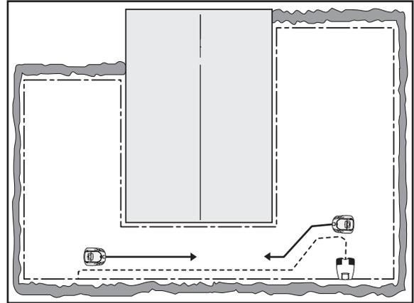
Avoid laying the wire at sharp angles. This can make it difficult for the mower to follow the guide wire.
