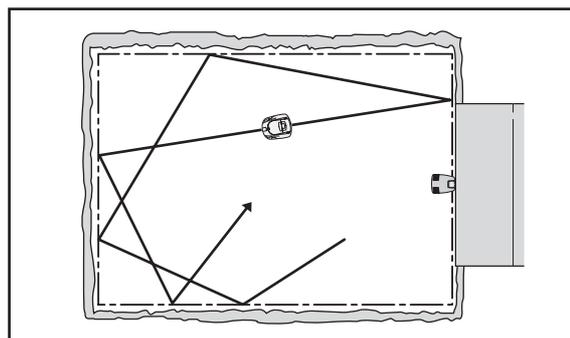
If Automower® enters an area where it senses the grass is longer than earlier, it can change the movement pattern. It can then mow in a square pattern to cover the area of longer grass more systematically.
