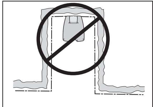
Avoid placing the charging station in a narrow passage (narrower than about 10 ft (3 metres)).
