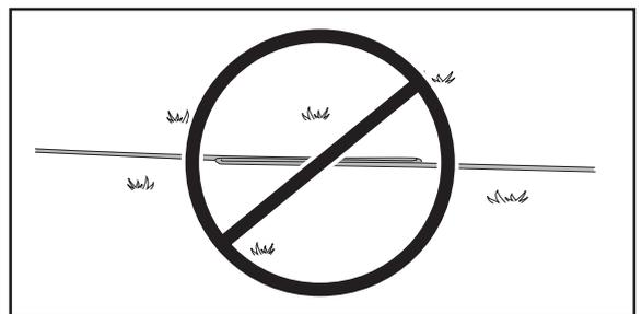
The boundary wire must not be crossed on the path to and from an island.
