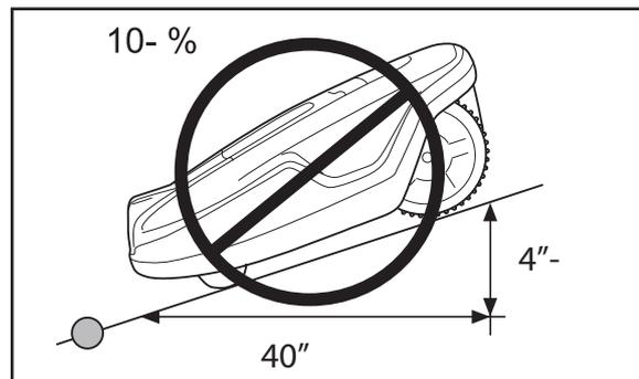
However, the boundary wire can be laid across a slope steeper than 10 % when there is an obstacle that Automower® can be permitted to collide with, for example, a fence or a dense hedge.
