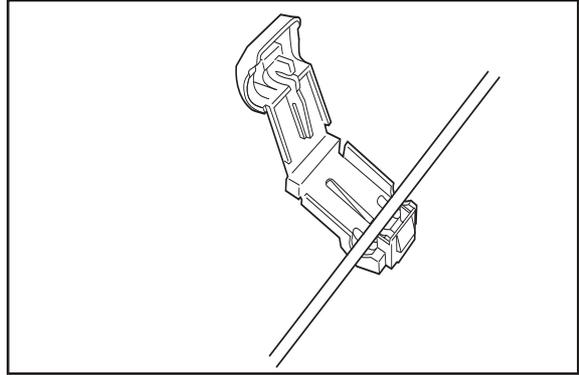
4. Press the connector together using a pair of pliers. Press until you hear a click.
