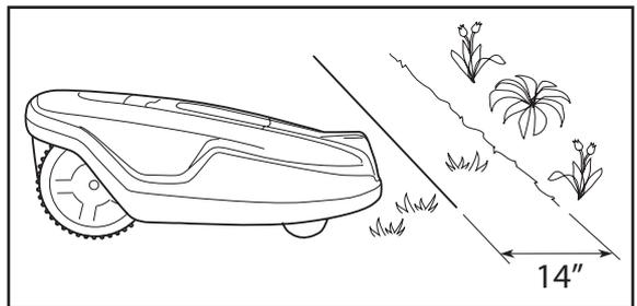
If the working area borders against a flat path or the like that lies level with the lawn, it is possible to allow Automower® to run a little over the path. The boundary wire should then be laid 4" (10 cm) from the edge of the path.
