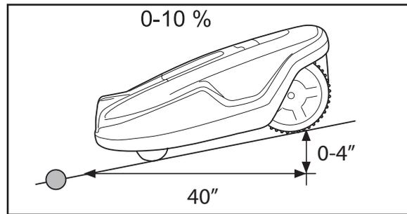
The boundary wire should not be laid across a slope that is steeper than 10 %. There is a risk of Automower® finding it difficult to turn there. The mower will then stop and show the fault message *Outside working area*. The risk is at its greatest in damp weather conditions, as the wheels can slip on the wet grass.
