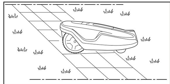
Note! Automower® must never run over a gravel path or similar material, which can damage the blades.
