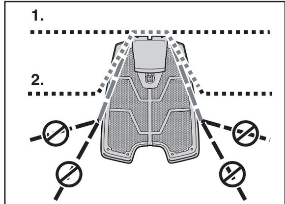
When connecting to the charging station, the right end of the boundary wire should be guided into the right-hand hole and the cable's left end in the left-hand hole.
