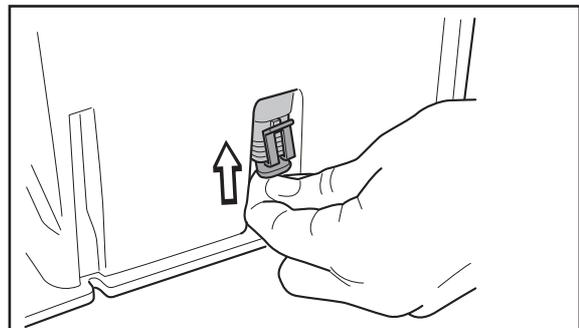
5. Connect the low voltage cable to the transformer.
