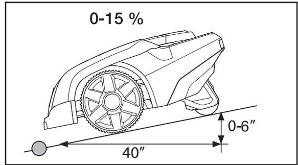
The boundary wire should not be laid across a slope that is steeper than 15%. There is a risk that the robotic lawnmower will find it difficult to turn there. The robotic lawnmower will then stop and the *Outside working area* fault message is displayed. The risk is at its greatest in damp weather conditions, as the wheels can slip on the wet grass
