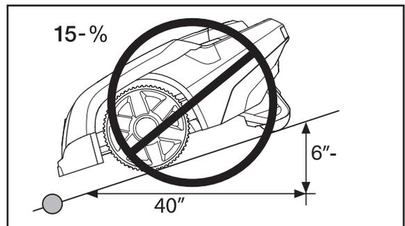
However, the boundary wire can be laid across a slope steeper than 15% if there is an obstacle that the robotic lawnmower is allowed to collide with, for example, a fence or a dense hedge.
