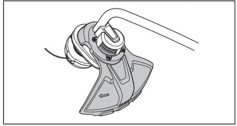
3. Replace the cutting attachment guard if it is damaged.
