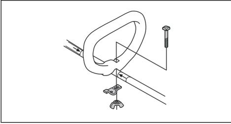
2. Make sure that the loop handle attaches between the arrows on the shaft.
