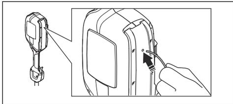
2. Pull out the line chute assembly.
