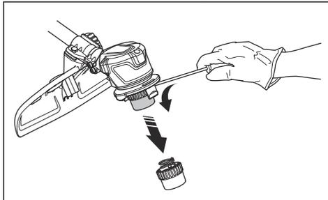
3. Remove the nut that holds the trimmer head and the drive disc.
