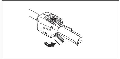
2. Push the power trigger lockout forward (A) and down. Hold the power trigger lockout against the handle (B) and make sure that it returns to its original position when you release it.
