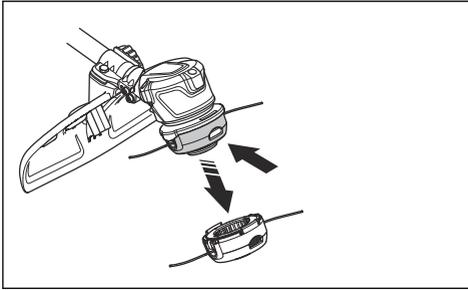
2. Pull out the line chute assembly.
