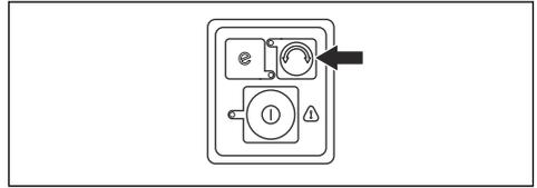
**Note:** It is easier to tap out the trimmer line to make it longer when the trimmer head turns clockwise.
