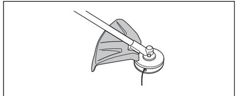
3. Replace the cutting attachment guard if it is damaged.
