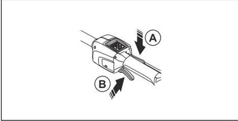
1. Make sure that the power trigger is locked when the lock is in its original position.
