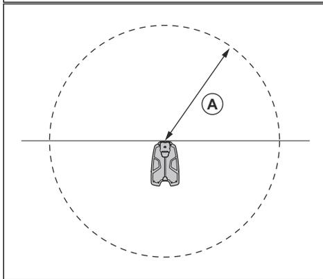
**Note:** The product uses the charging station signal to search for the charging station when it is in the docking area.
