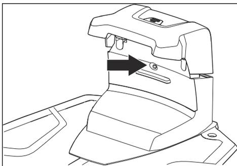
2. If the indicator LED lamp does not have a green light, do a check of the installation. Refer to *To install the charging station on page 15* and *LED indicator lamp on the charging station on page 34*.
