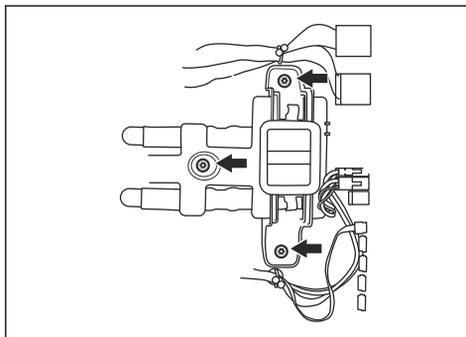
9. Disconnect the batteries connection from the main circuit board.
