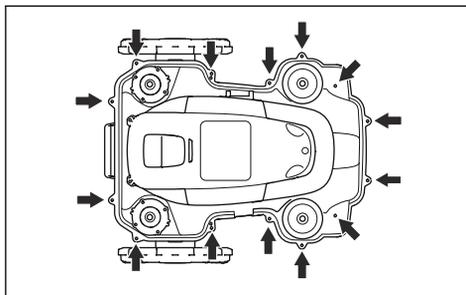
5. Lift the rear edge of the top section of the chassis.
