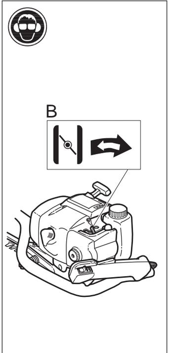
Press the machine body against the ground using your left hand (NOTE! Do not use your foot). Grip the starter handle with your right hand and slowly pull the starter cord out until you feel some resistance, (the starter hooks grip) now quickly and powerfully pull the cord.
