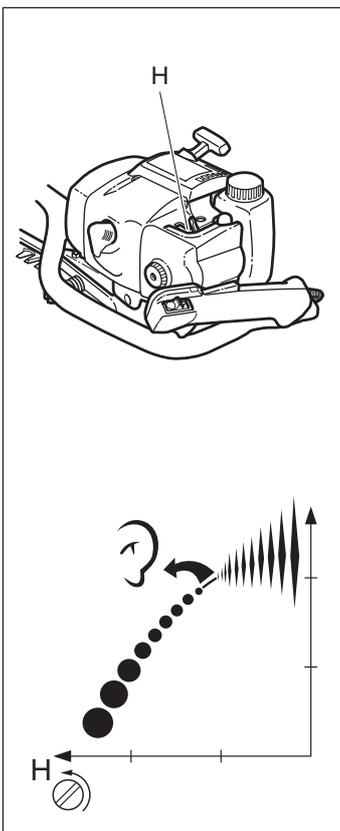
The high speed needle is adjusted correctly when the machine "splatters" a little. If the machine smokes heavily at the same time as it "splatters" heavily the adjustment is too rich.
