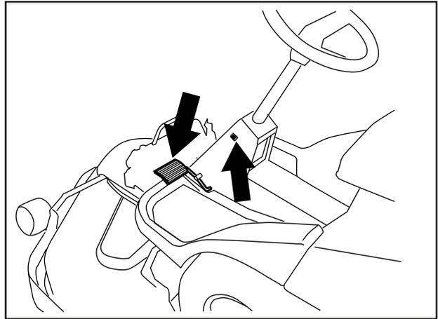
3. Lift up the unit using the lifting lever.
