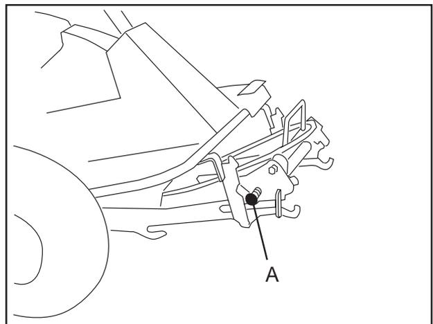
1. Fit the unit in the attachment frame's outer hooks.
