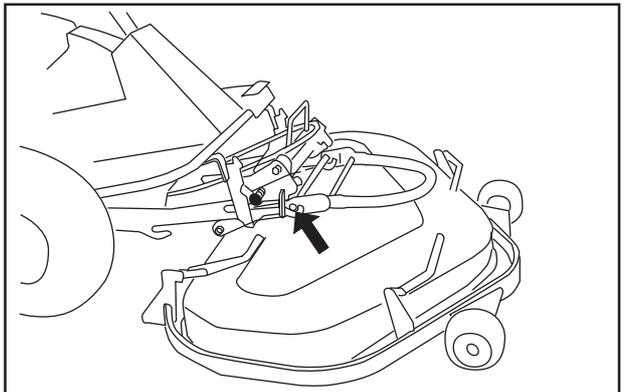
2. Pull out the catch (A) and release the hook guard by sliding its handle backwards.
