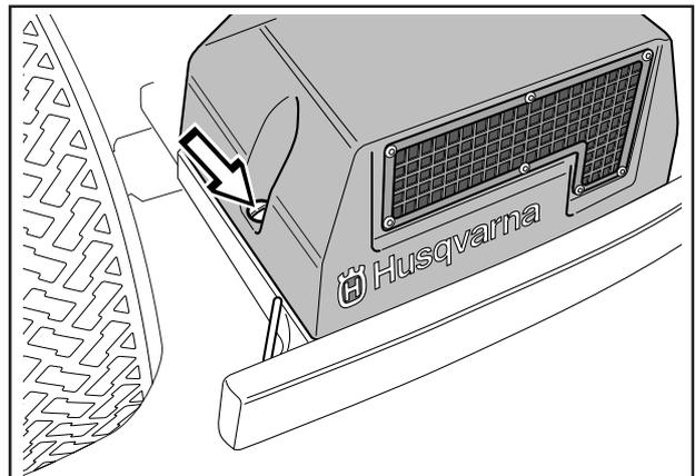
2. Screw off the oil canister cap and top up with engine oil SAE 10W/30, class CD-CF, until the oil level reaches the MAX marking. Screw the oil canister cap back on, and fit the transmission cover.
