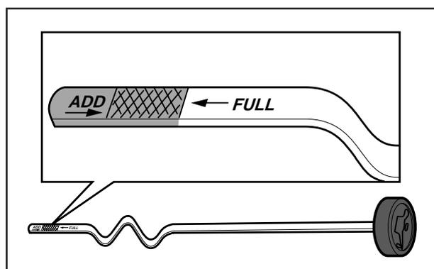
The oil is filled in the same hole as the dip stick.
