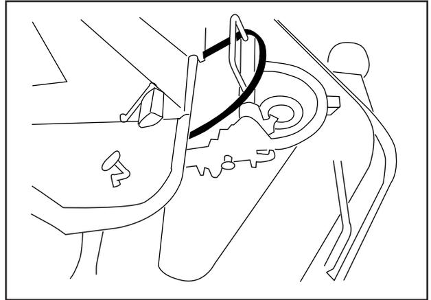
3. Fit the steering plate under the support wheel and tighten the bolts using two 13 mm socket spanners.
