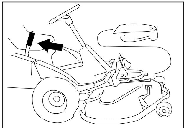
5. Remove the belt adjuster's spring.
