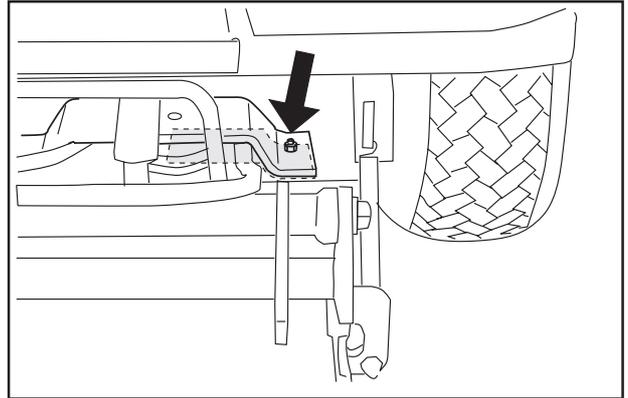
2. Unhook the spring on the blade brake.
