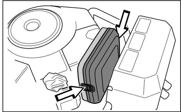
3. Release and remove the wing-nut in the centre of the air filter and lift off the paper filter with pre-filter.
