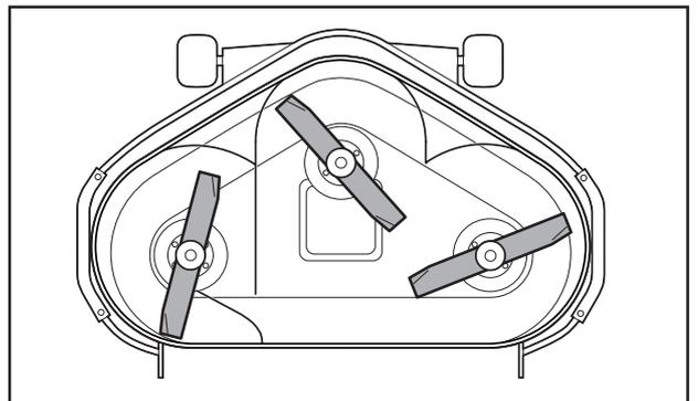
*Cutting unit with rear ejector*
