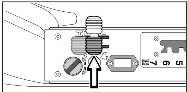
3. If the engine is cold move the choke lever backwards to its end position.
