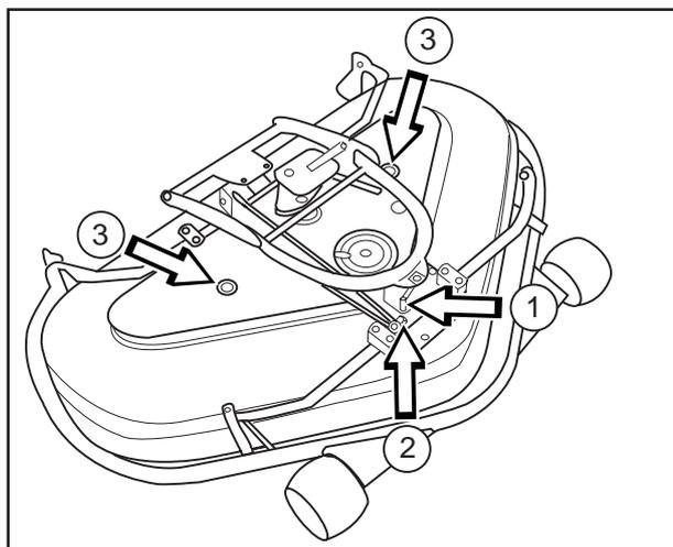
2. Loosen the spring that tensions the V-belt and pry off the belt.
