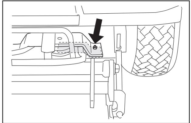
4. Hook on the spring for the blade brake.
