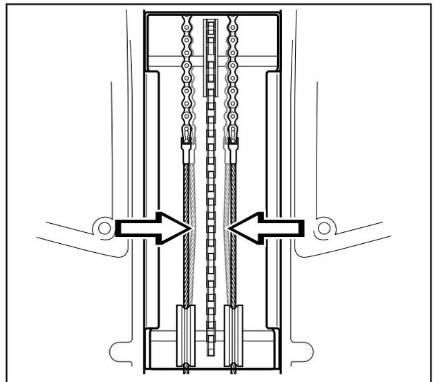
3. When necessary the wires can be tensioned by tightening the adjusting nuts (one on each side of the machine). Do not tension the wires too tightly, they should only be *tightened up* to the steering rim. Check the wire tension on completion of the adjustment as per item 2.
