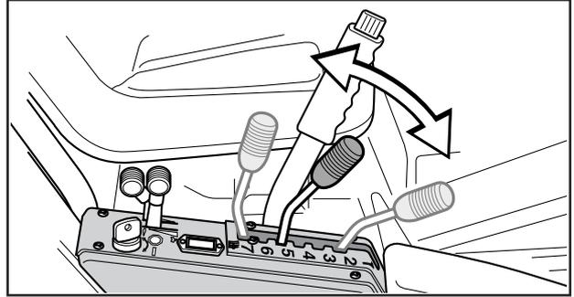
4. Push in the lock button on the lift lever and lower down the cutting unit.
