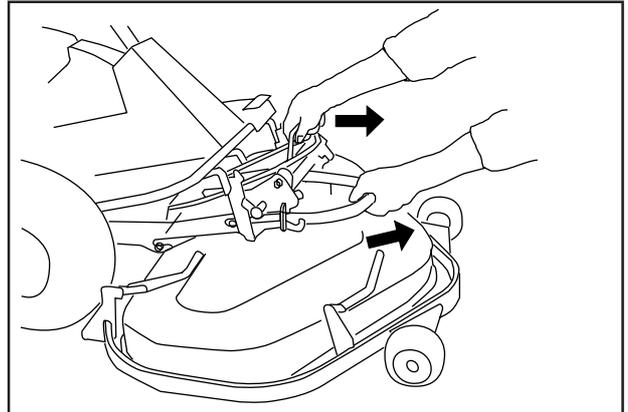
11. Pull out the unit so that it engages in the outer hooks.
