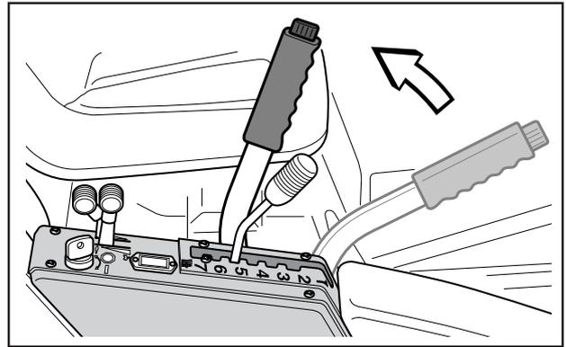
*Lifting of the cutting unit*
