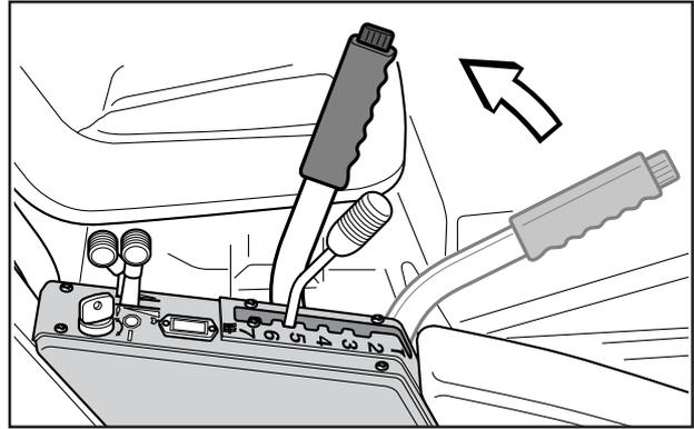
2. Move the throttle control to the MIN. position.
