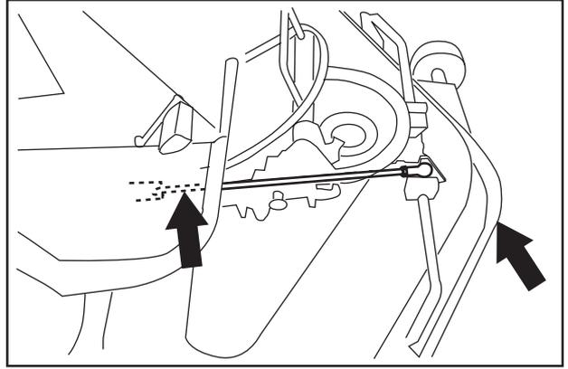
10. Pull the handle and unit simultaneously. Release the handle when the unit has come out a little.
