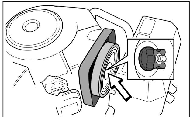
4. Pull off the foam plastic pre-filter from the paper filter and wash clean in mild detergent.
