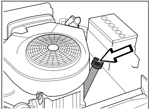
The oil level should lie between the markings on dip stick. If the level approaches the ADD mark, top up with oil to the FULL mark on the dip stick.
