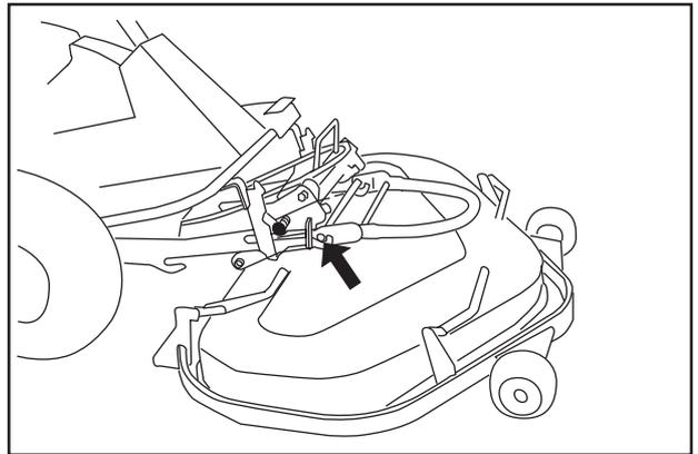
13. Pull the handle so that the hook guard locks. Check that the catch (A) is in its loaded position.
