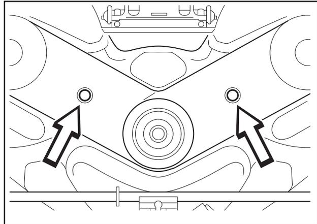
3. Loosen the nuts on the eccentric plate and turn this away.
