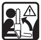
Contact with the guide bar tip can cause the saw to be thrown violently upwards and backwards (kickback), which can result in serious injury.
