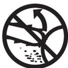
Avoid contact between the guide bar tip and any object.
