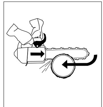
7 Follow the instructions on sharpening and maintaining your bar and chain. When you replace the bar and chain use only combinations that are recommended by us. See the sections on "Cutting equipment" and "Technical data".
