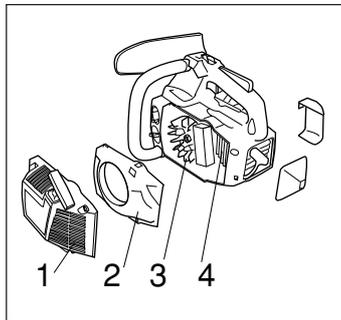
Clean the cooling system with a brush once a week, more often in demanding conditions. **A dirty or blocked cooling system results in the saw overheating which causes damage to piston and cylinder.**
