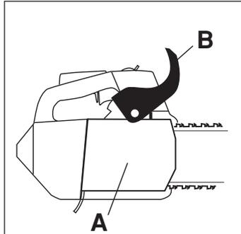
The brake is applied when the front hand guard (B) is pushed forwards.
