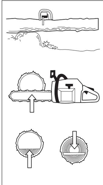
A Start by cutting from below (about 1/3 of the way through).
