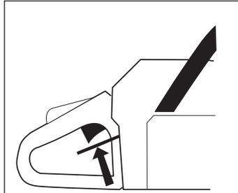
2 Press the throttle lock and make sure it returns to its original position when you release it.
