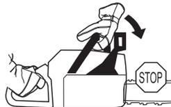
• Place the saw on the ground and hold the rear handle down with your right foot. Grasp the front handle firmly using your left hand. Make sure the chain saw is steady and the chain is not touching the ground. Then grasp the starter handle with your right hand and pull the starter cord. Never wrap the starter cord around your hand.
