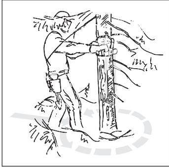
Remove any undergrowth from the base of the tree and check the area for obstacles (stones, branches, holes, etc.) so that you have a clear path of retreat when the tree starts to fall. Your path of retreat should be roughly 135 degrees behind the intended felling direction.
