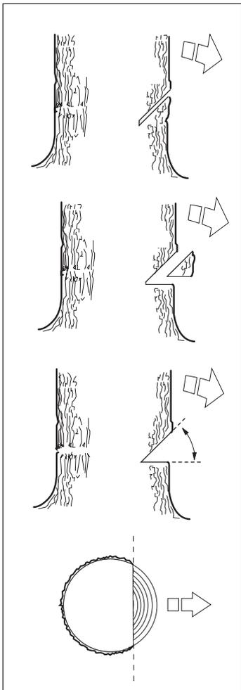
Next make the BOTTOM CUT so that it finishes at the end of the TOP CUT.
