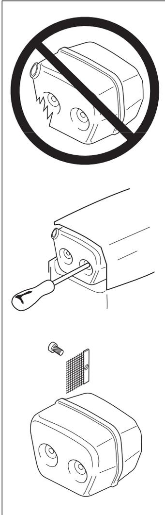
Regularly check that the muffler is securely attached to the chain saw.
