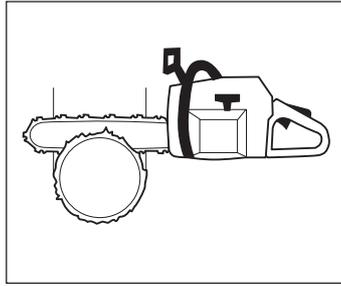
There are methods for felling trees with a diameter larger than the bar length. However these methods involve a much greater risk that the kickback zone of the bar will come into contact with the tree.
