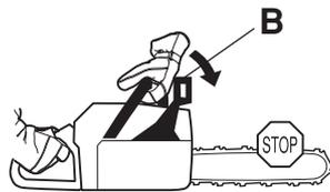
The brake is applied when the front hand guard (B) is pushed forwards.
