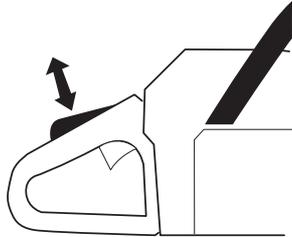
3 Check that the throttle control and throttle lock move freely and that the return springs work properly.
