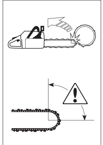
Kickback always occurs in the cutting plane of the saw. Normally the saw and bar are thrown backwards and upwards towards the user. However the saw may move in a different direction depending on the way it was being used when the kickback zone of the bar touched the object.
