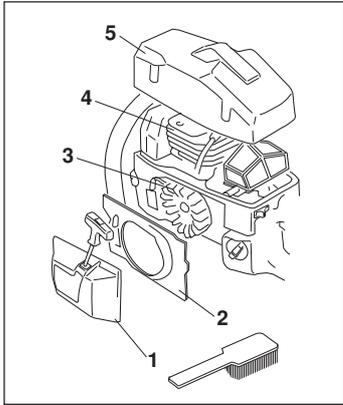
Clean the cooling system with a brush once a week, more often in demanding conditions. **A dirty or blocked cooling system results in the saw overheating which causes damage to piston and cylinder.**
