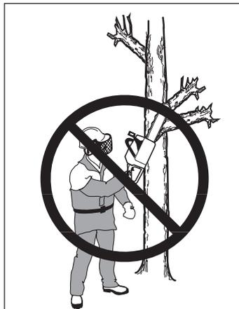
5 In order to keep control of your saw, always maintain a firm foothold. Never work on a ladder, in a tree or any other insecure support.
