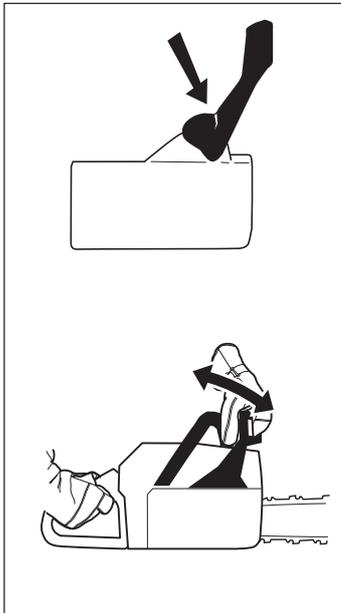
B Move the front hand guard forwards and back to make sure it runs freely and that it is securely anchored to the clutch cover.
