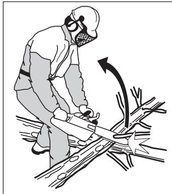
4 Never use the saw above shoulder height and try not to cut with the tip of the bar.
