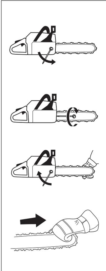
The position of the chain tensioning screw varies from model to model. See the "What is what" section to find out where it is on your saw.
