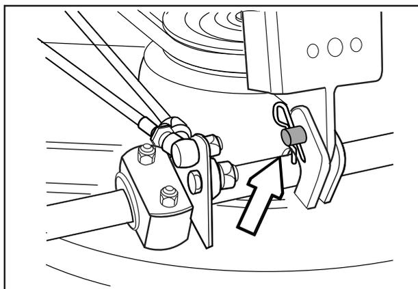
4. Press down the frame and insert the pin. Fit the drive belt around the drive wheels of the cutting unit.
