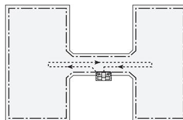
The area in front of the charging station should be as open as possible. Don't put the charging station in a "pocket". We recommend that the charging station is placed somewhere along a straight part of the boundary wire rather than in a corner.
