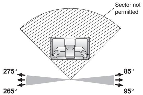
The angles at which the Auto Mower sets off can be restored to the default settings by keying in \* 36 #.
