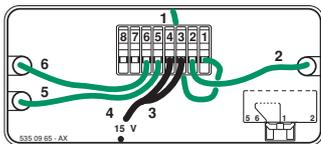
Use the tool supplied to connect the six wires to the terminal block. See drawing.
