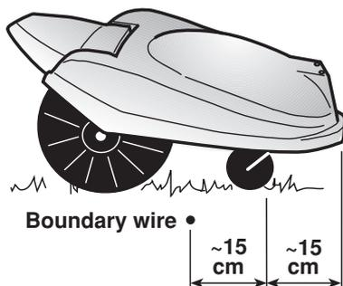
The nose of the mower projects no more than 30-35 cm over the boundary wire and the front wheel projects 10-15 cm over the boundary wire. The Auto Mower mows around 12-17 cm over the boundary wire.
