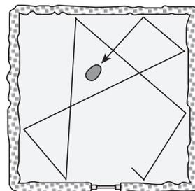
If the Auto Mower enters an area where it senses that the grass is longer than where it has just been, it can start to mow systematically. It then mows in a spiral pattern, mowing the area that has longer grass than the surrounding area. After this it returns to the random principle.
