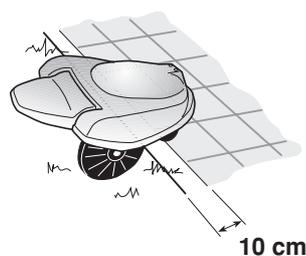
Long narrow passages (more than 2 meters in length) should be at least 2 m wide, i.e. leaving 140 cm between the wires, to give the Auto Mower enough space to make its way through. See the illustration. Shorter passages (less than 1 meter long) should be at least 1.2 m wide.
