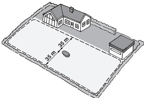
When the Auto Mower's working area borders, e.g. collections of water, driveways and pathways, etc. the boundary wire must be supplemented with a number of posts, edging or a fence with a height of at least 15 cm. This is an additional safety measure to prevent the Auto Mower from running outside of its working area.
