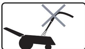
Never use a high-pressure jet or even running water to clean the Auto Mower.
