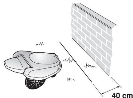
Where the lawn finishes with a ditch or a small rise, such as curb stones (max. 5 cm high), lay the boundary wire 30 cm inside the edge of the working area. This ensures that the wheels will not fall into the ditch or ride up on the curb stones.
