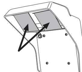
Remove corrosion from the Auto Mower charging pins and charging station contact plates if necessary, e.g. after winter storage or if there is a problem with charging. Use a fine abrasive cloth to clean the charging pins and contact plates.
