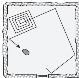
Initially the Auto Mower works for a few hours to get an idea of the average length and thickness of the grass. Only then does it start working systematically.
