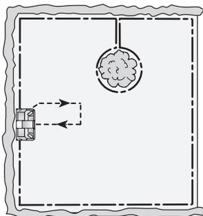
The boundary wire must be no longer than 500 metres. The distance between the Auto Mower and the nearest part of the boundary wire must not exceed 35 metres anywhere in the working area.
