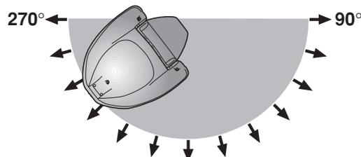
The mower normally leaves the charging station at a random angle within the range 90–270° (see diagram).
