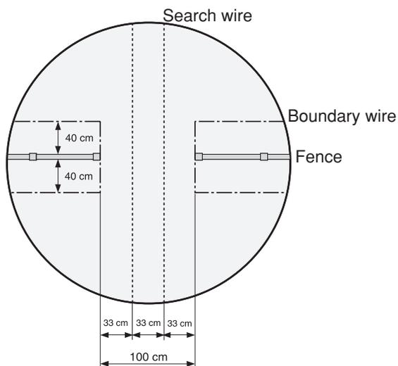
Since the Auto Mower follows the path of the search wire, it must be laid at least 40 cm away from any obstacle to prevent the Auto Mower from bumping into anything on its way to the charging station.
