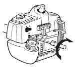
IMPORTANT! If the idle speed cannot be adjusted so that the cutting attachment stops, contact your dealer/service workshop. Do not use the machine until it has been correctly adjusted or repaired.
