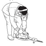
Push the choke control back to its original position as soon as the engine fires, and continue trying to start until the engine starts. When the engine starts, quickly apply full throttle to automatically disengage the start throttle setting.
