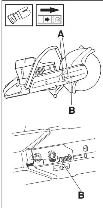
**IMPORTANT INFORMATION! A new drive belt should be tensioned after using one tank of fuel.**
