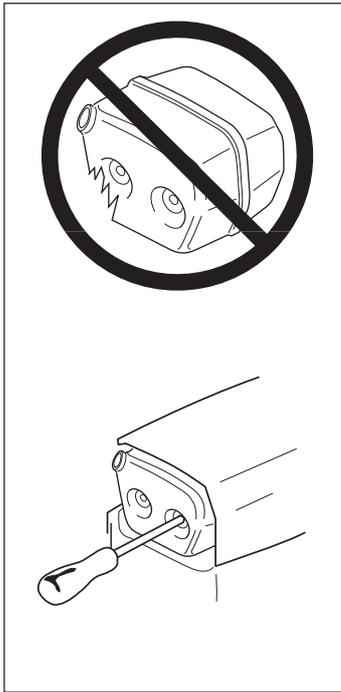
Check regularly that the muffler is secured to the engine body.
