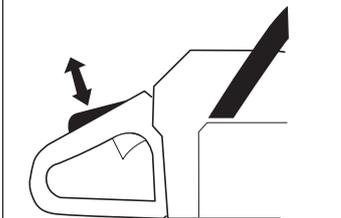
3 Check that the throttle control and throttle lock move freely and that the return springs work properly.
