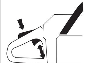
4 Start the power cutter and apply full throttle. Release the throttle control and check that the blade stops and remains stationary. If the blade rotates when the throttle is on idle setting you should check the carburettor idle adjustment. See the section on "Maintenance".
