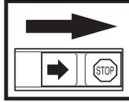
Switch off the engine by moving the stop switch to the STOP position before carrying out any checks or maintenance.
