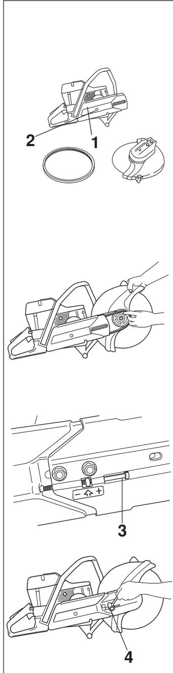
Feed the drive belt over the pulley on the cutting head.
