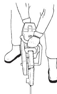
Check that the anti-vibration elements are securely mounted between the engine unit and the handle system.
