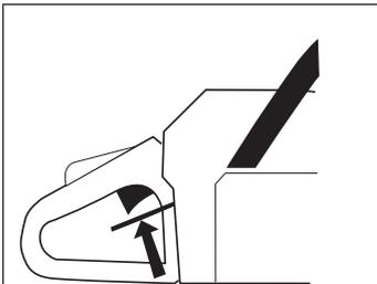
2 Press the throttle lock and make sure it returns to its original position when you release it.
