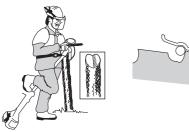
The filing angle is 15°. File alternate teeth to the right and those in between to the left. If the blade has been heavily pitted by stones it may be necessary to dress the top edges of the teeth with a flat file, in exceptional cases. If so, this should be done before filing with a round file. The top edges must be filed down by the same amount for all the teeth.
