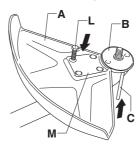
Screw on the trimmer head/plastic blades (H) in the opposite direction to the direction of rotation.
