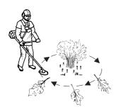
Avoid cutting with the area of the blade between the 12 o'clock and 3 o'clock positions.
