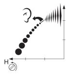
You have now run the machine at settings of H =±0, H=+1/4, H=+1/2 relative to the basic settings. At full throttle the engine has sounded different for each setting. The H-jet is correctly adjusted when the machine burbles a little. If the machine "screams" then the machine is set too lean. If the muffler emits a lot of smoke and the machine burbles a lot then the setting is too rich. Turn the H-jet clockwise until the setting sounds right
