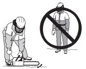
Place the chain saw on the ground and hold the rear handle down with your right foot. Grasp the front handle firmly using your left hand. Make sure the chain saw is steady and the chain is not touching the ground or other objects. Then grasp the starter handle with your right hand and pull the starter cord. **Never twist the starter cord around your hand.**
