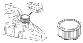
• The filter can be cleaned more thoroughly by washing it in water and detergent.
