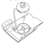
Remove the recoil spring from inside the pulley by tapping the pulley lightly with its inside face downwards against a work bench or the like. If the spring pops out during fitting, wind it up again, working from the outside in towards centre.  Lubricate the recoil spring with light oil. Fit the pulley and tension the recoil spring.
