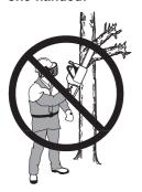
5 You must have a steady stance in order to have full control over the chain saw. Never work standing on a ladder, in a tree or where you do not have firm ground to stand on.
