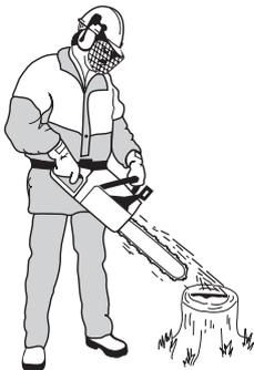
If the chain lubrication is not working:
