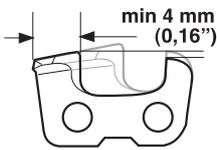
When the length of the cutting teeth has worn down to only 4 mm the chain must be replaced.
