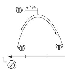
Turn the low speed jet L clockwise until it stops. If the engine accelerates poorly or idles unevenly, turn the low speed jet L anticlockwise until good acceleration and idling are achieved.
