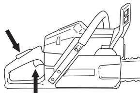
Push in the choke control as soon as the engine fires and make repeated starting attempts. Immediately press and release the throttle when the engine starts. That will disengage the throttle latch.
