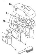
Clean the cooling system with a brush once a week, more often in demanding conditions. A dirty or blocked cooling system results in the machine overheating which causes damage to the piston and cylinder.
