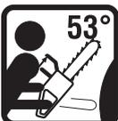
Measured maximum kickback value without triggering the brake, for the bar and chain combination on the label.
