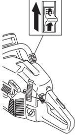
When the switch is pushed upwards, the heat is switched on. When the switch is pushed downwards, the heat is switched off.
