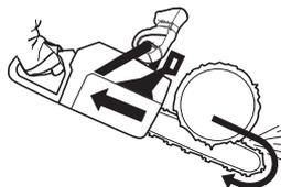
Unless the user resists this pushing force there is a risk that the chain saw will move so far backwards that only the kickback zone of the bar is in contact with the tree, which can lead to a kickback.
