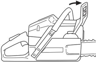
**Starting:** The chain brake should be activated when starting the chain saw. Activate the chain brake by pushing the front hand guard forwards.
