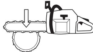
Finish by cutting from below so that the two cuts meet.
