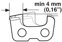
When the length of the cutting teeth has worn down to only 4 mm (0,16 inch) the chain must be replaced.
