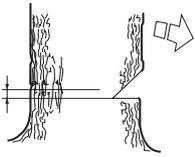
Use full throttle and bring the bar and chain slowly into the tree. Make sure the tree does not start to move in the opposite direction to your intended felling direction. Drive a wedge or breaking bar into the cut as soon as it is deep enough.
