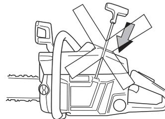
Push in the choke control as soon as the engine fires and make repeated starting attempts. Immediately press and release the throttle when the engine starts. That will disengage the throttle latch.
