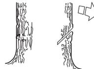
Next make the bottom cut so that it finishes exactly at the end of the top cut.
