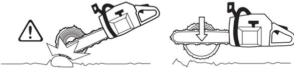
If it is possible (can you turn the log?) stop cutting about 2/3 of the way through the log.
