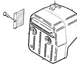
Some mufflers are equipped with a special spark arrester mesh. If your machine has this type of muffler, you should clean the mesh at least once a week. This is best done with a wire brush.
