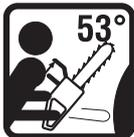
Measured maximum kickback value without triggering the brake, for the bar and chain combination on the label.
