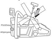
Push in the choke control as soon as the engine fire and make repeated starting attempts. Immediately press and release the throttle when the engine starts. That will disengage the throttle latch.
