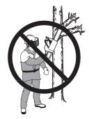
In order to keep control of your saw, always maintain a firm foothold. Never work on a ladder, in a tree or on any other insecure support.
