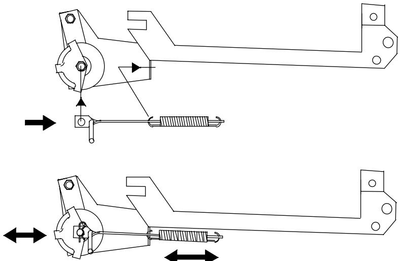
**8 C**Cable operated clutch,
