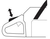
• Check that the throttle control and throttle lock move freely and that the return springs work properly.
