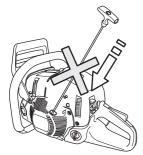
Note! Pull the front hand guard towards the front handle. The chain brake is now disengaged. Your saw is ready for use.
