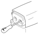
Some mufflers are equipped with a special spark arrestor mesh. If your machine has this type of muffler, you should clean the mesh at least once a week. This is best done with a wire brush. A blocked mesh will cause the engine to overheat and may lead to serious damage.
