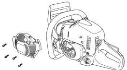
• Pull out the cord approx. 30 cm (12 inches) and hook it into the notch in the rim of the pulley. Release the recoil spring by letting the pulley rotate slowly backwards.
