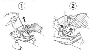
Undo the screw in the centre of the pulley and remove the pulley. Insert and fasten a new starter cord to the pulley.
