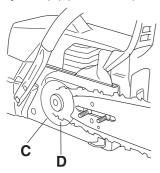
The front hand guard is not designed solely to activate the chain brake. Another important feature is that it reduces the risk of the chain hitting your left hand if you lose grip of the front handle.
