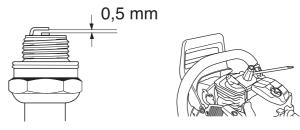
Note! Always use the recommended spark plug type! Use of the wrong spark plug can damage the piston/cylinder. Check that the spark plug is fitted with a suppressor.
