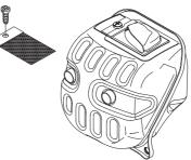
The muffler is designed to reduce the noise level and to direct the exhaust gases away from the operator. The exhaust gases are hot and can contain sparks, which may cause fire if directed against dry and combustible material.
