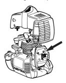
Some mufflers are equipped with a special spark arrestor mesh. If your machine has this type of muffler, you should clean the mesh at least once a week. This is best done with a wire brush. On mufflers without a catalytic converter the mesh
