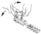
Grasp the handle on the angle stop, adjust to the desired angle and then tighten the knob.
