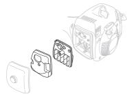
An oiled foam plastic filter (available as an accessory) must be used if the machine is operated in extremely dusty conditions. See instructions under the heading Oiling the air filter.
