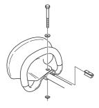
5 Now make a final adjustment to give yourself a comfortable working position. Tighten the screw. CAUTION! The loop handle and hand guard must not be fitted behind the arrow marked on the shaft.
