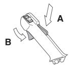
Make sure the throttle control is locked at the idle setting when the throttle lock is released.
