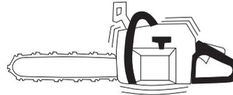
Make sure the vibration damping units are securely attached to the engine unit and handle unit.
