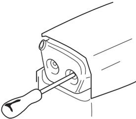
A blocked mesh will cause the engine to overheat and may lead to serious damage.
