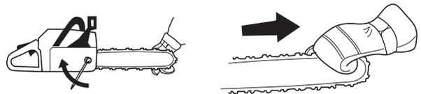
The position of the chain tensioning screw on our chain saws varies from model to model. See instructions under the heading What is what? to find out where it is on your model.
