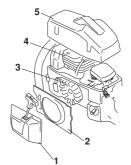
Clean the cooling system with a brush once a week, more often in demanding conditions. A dirty or blocked cooling system results in the machine overheating which causes damage to the piston and cylinder.
