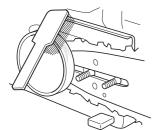
Regularly check that the brake band is at least 0.6 mm (0,024 inch) thick at its thinnest point.
