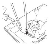
Undo the screw in the centre of the pulley and remove the
