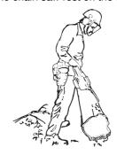
Keep the trunk between you and the chain saw as you move along the trunk.
