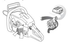
IMPORTANT! In order to maintain operation of the centrifugal cleaning system it must be regularly maintained. Clean the air intake to the starter, the fins on the flywheel, the space around the flywheel, inlet pipe and carburetor compartment.
