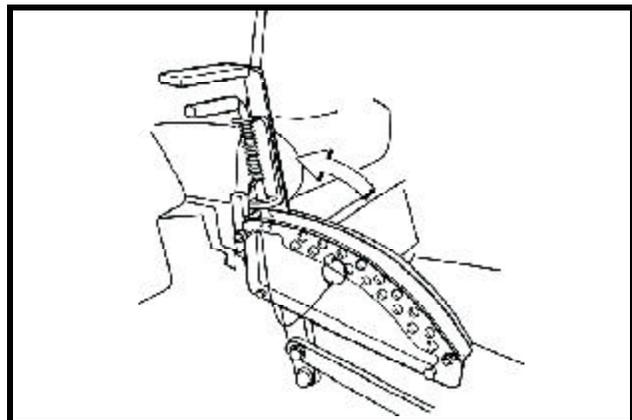
*Raise the mower deck - 27.5 HP engine*
