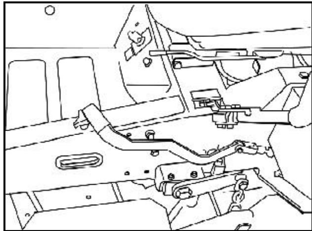
Parking brake in the disengaged position
