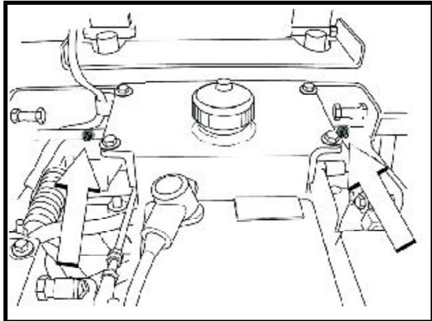
*Lubricating the steering control shafts*
