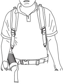
Tighten the side straps so that the pressure is evenly distributed across the shoulders.
