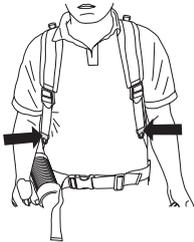
Place the hip strap over the hip and not too far down on the stomach. Tighten the hip strap so that you feel the weight of the blower resting on your hip.
