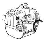
Apply full throttle and turn the high speed jet H very slowly clockwise until the engine slows down. Then turn the high speed jet H very slowly anticlockwise until the engine starts to run unevenly. Now turn the high speed jet H slowly clockwise a little way until the engine runs smoothly.
