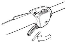
Press the throttle lock and make sure it returns to its original position when you release it.
