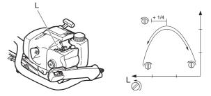
**CAUTION!** If the blades move while the engine is idling the T screw should be turned anti-clockwise until they stop.
