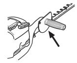
Check that the hand guard is fitted correctly. Check that the hand guard is undamaged.
