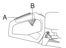
Make sure the throttle control is locked at the idle setting when the throttle lock is released.
