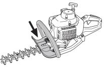
Check that the hand guard is fitted correctly. Check that the hand guard is undamaged.
