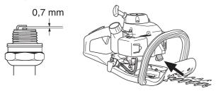
**CAUTION!** Always use the recommended spark plug type! Use of the wrong spark plug can damage the piston/cylinder. Check that the spark plug is fitted with a suppressor.
