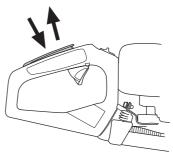
Check that the throttle control and throttle lock move freely and that the return springs work properly.
