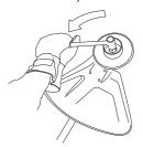
Fit the bottom half of the trimmer head (K) to the cover (I) by pressing them together, with the cut-outs on the bottom half aligned with the catches on the cover.
