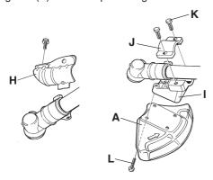
CAUTION! Always use the recommended guard for the cutting attachment you are using. See chapter on Technical data.
