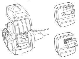
Some mufflers are equipped with a special spark arrestor mesh. If your machine has this type of muffler, you should clean the mesh at least once a week. This is best done with a wire brush.
