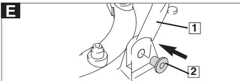
1. Fit the lower handle (E1) to the deck with the lower handle pin (E2) as illustrated in Fig E.
