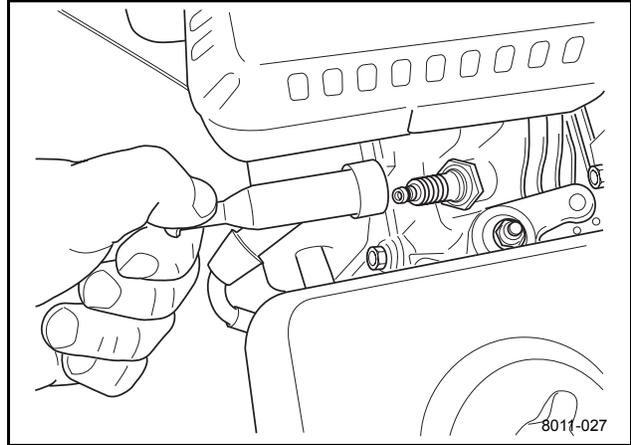
*Remove the spark plug cable*
