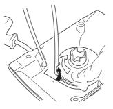
Undo the screw in the centre of the pulley and remove the pulley. Insert and fasten a new starter cord to the pulley. Wind approx. 3 turns of the starter cord onto the pulley. Connect the pulley to the recoil spring so that the end of the spring engages in the pulley. Fit the screw in the center of the pulley. Insert the starter cord through the hole in the starter housing and the starter handle. Make a secure knot in the end of the starter cord.
