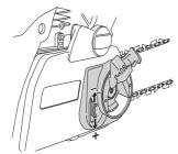
The chain is correctly tensioned when it does not sag from the underside of the bar, but can still be turned easily by hand. Hold up the bar tip and tighten the bar clutch by turning the knob clockwise.
