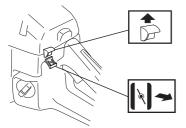
If the machine is fitted with an air purge (A): Press the air purge repeatedly until fuel begins to fill the bulb. The bulb need not be completely filled.
