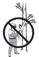
5 In order to keep control of your saw, always maintain a firm foothold. Never work on a ladder, in a tree or on any other insecure support.
