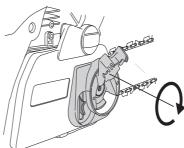
· Fold the knob back in to lock the tensioning.
