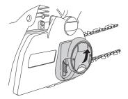
• Turn the knob anti clockwise to loosen the bar cover.
