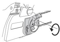
• Adjust the tension on the chain by turning the wheel down (+) for tighter tension and up (-) to loosen the tension.
