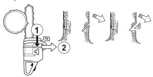
The directional cuts should run 1/4 of the diameter through the trunk and the angle between the top cut and bottom cut should be  $45^{\circ}$ .
