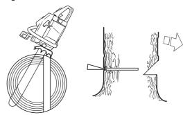
Finish the felling cut parallel with the directional cut line so that the distance between them is at least 1/10 of the trunk diameter. The uncut section of the trunk is called the felling hinge.
