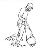
Keep the trunk between you and the chain saw as you move along the trunk.
