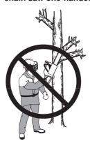
5 You must have a steady stance in order to have full control over the chain saw. Never work standing on a ladder, in a tree or where you do not have firm ground to stand on.
