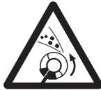
The operator of the machine must ensure, while working, that no persons or animals come closer than 15 metres.
