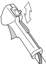
Check that the throttle control and throttle lockout move freely and that the return springs work properly.
