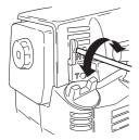
Note that the engine should not be under load when you adjust the high speed jet H. You should therefore remove the cutting attachment, nut, support flange and drive disc before adjusting the high speed jet H.
